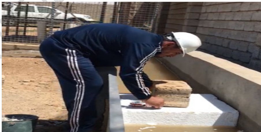
Fig. 5. Weight on the Floating Bridge test
