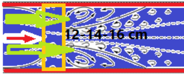
Fig.14. Flow through a bridge opening
