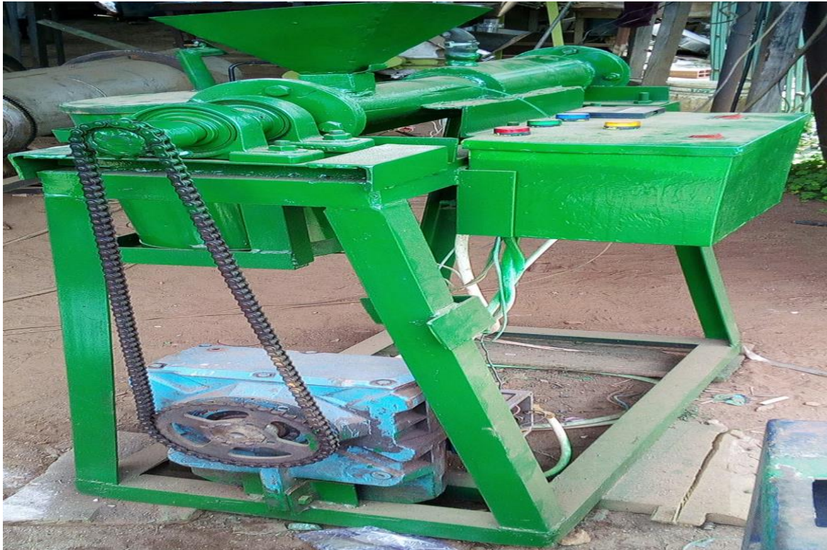
Plate 2: Pictorial View of the Modified Extruder
