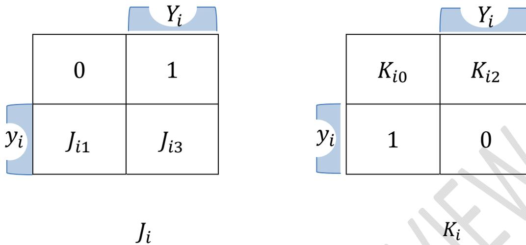
**Fig. 4.** The general solution for  $J_i$  and  $K_i$  in terms of  $Y_i$  and  $y_i$ . The atomic components  $J_{i1}$ ,  $J_{i3}$ ,  $K_{i0}$  and  $K_{i2}$  are not specified and remain to be arbitrary binary constants.
