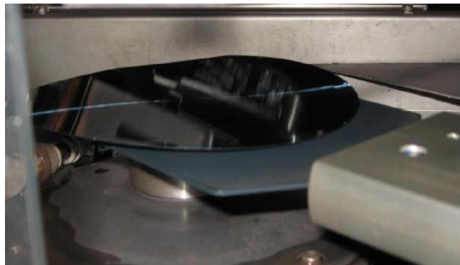
Fig. 7. Vacuum error on the robot arm
