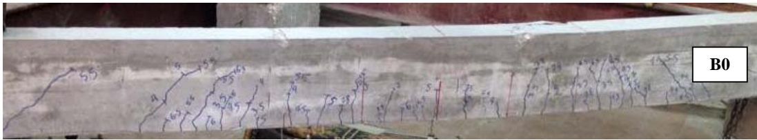
Fig. 6a. Flexural failure for B0 beam specimen without spliced
