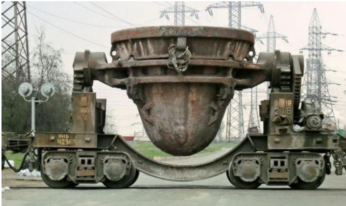
Figure 9 – Slag chalice on a slag-transfer platform (the volume is 15m 3 , the height is 3240 mm, the diameter is 3740 mm)
