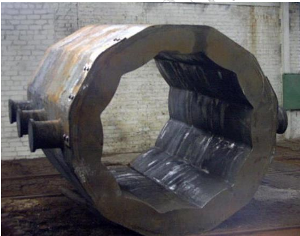
Figure 8 – A through mold for a forging casting (the weight is 42 tons, the wall thickness is 350 mm)
