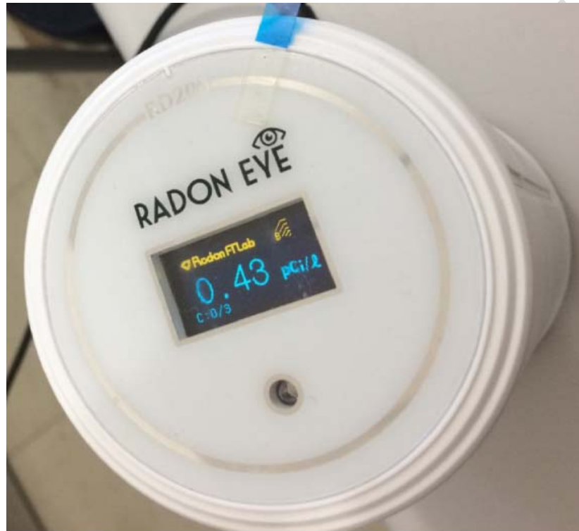
Fig 3 – Top view of Radon Eye RD200 ionization chamber used for monitoring radon gas [11]
