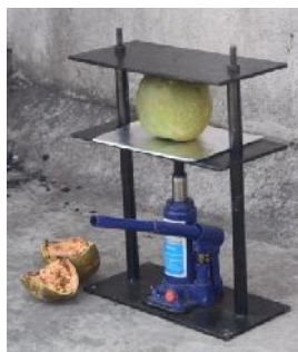
Fig 8: Diagonal view of Shell cracker
