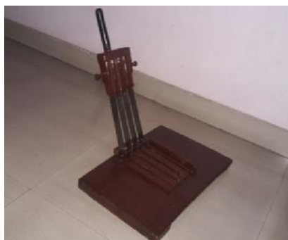
Fig 4: Diagonal view of Veg-multi-slicer
