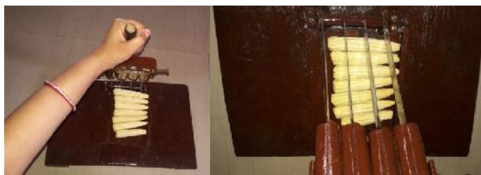
Fig 5: Cutting multiple baby corns with veg-multi-slicer
