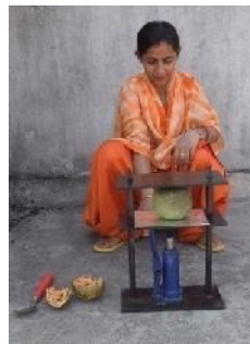
Fig 10: Worker using shell cracker
