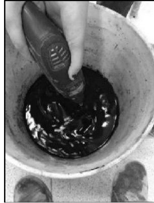
Figure 2. Dispersion of MWCNTs
