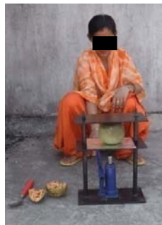
Fig 10: Worker using shell cracker
