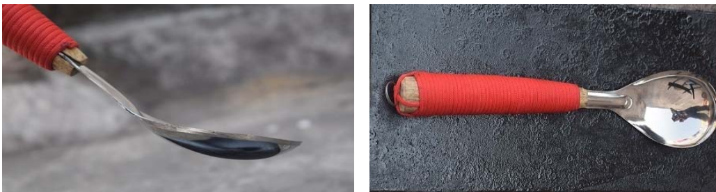
Fig. 1: Side and front view of Pulp extractor
