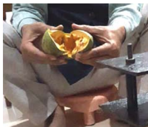
Fig 12: Separating shells after cracking the shells with Shell cracker
