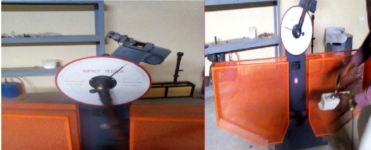
123 124 Fig. 1: Impact Testing Setup
