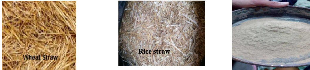
FIG. 2 Wheat and rice straw ash before and after grinding
