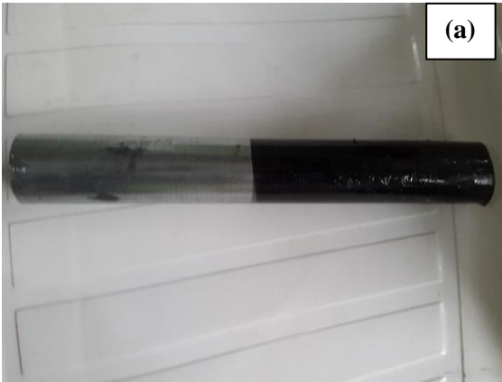
Fig. 8(a): Showing a half-coated pipe tested for coating flaws (b) Result of test galvanized pipe with coating flaws
