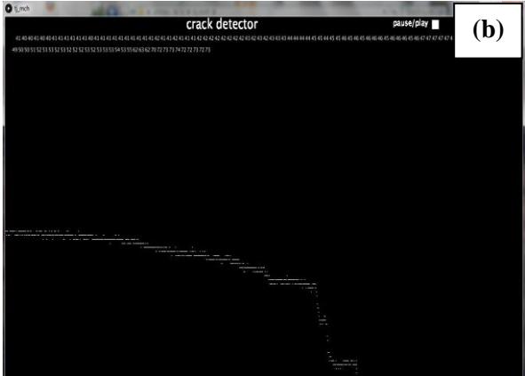
Fig. 8(a): Showing a half-coated pipe tested for coating flaws (b) Result of test galvanized pipe with coating flaws
