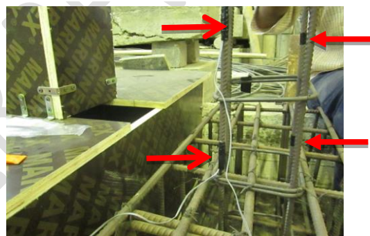
Figure 3: Strain Gauge locations
