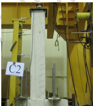
Figure 6: The cracks of C2 column under the lateral loads
