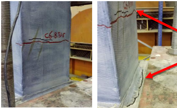
Figure 13: The cracks of C2C1 column at failure under the lateral load. Separation of the fiber is noticed
