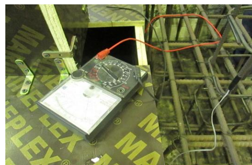
Figure 4: Calibration of the strain gauges
