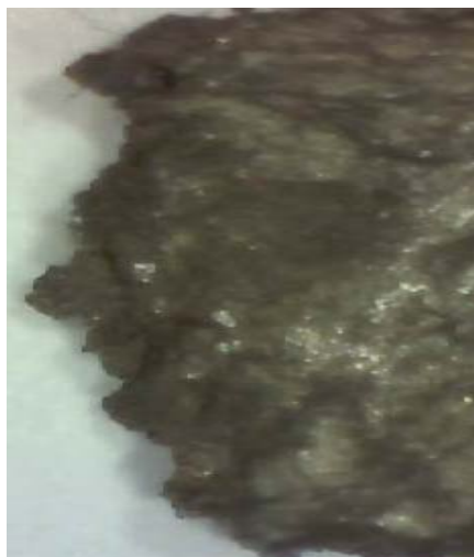
Figure 1. \text{Pb:Sn:Bi} alloy with carbon particles
