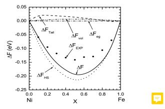
Figure 4: Energy of formation for  $Fe_xNi_{1-x}$  liquid binary alloys as a function of concentration.Lines denote theoretical results and closed circles experimental data. All the symbols are defined in the text.
