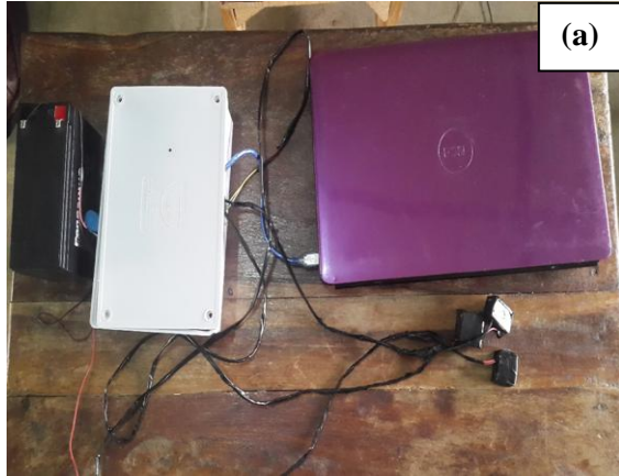
Fig. 4: (a) Complete set-up of an eddy current test device (b) The Micro-controller
