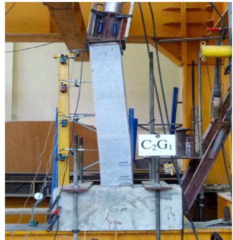
Figure 9: The cracks of column C2G1 at failure under the ultimate axial load
