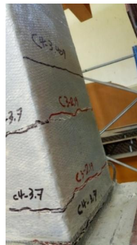
Figure 27: Crack Pattern for Confined Columns
