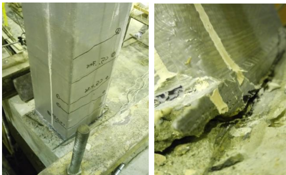
Figure 11: The cracks of C2G2 column at failure under the lateral load. Separation of the fiber is
