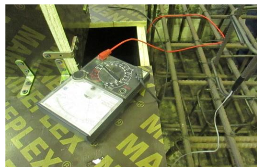
Figure 4: Calibration of the strain gauges
