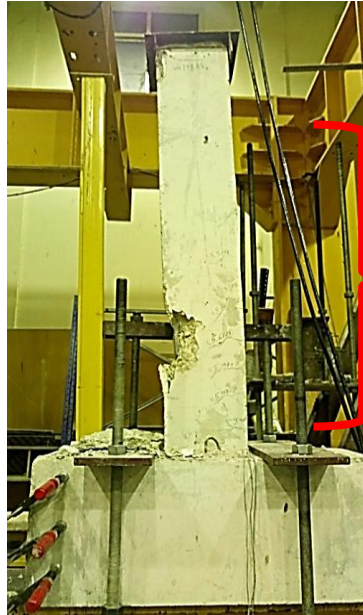
Figure 26: Crack Pattern for Unconfined Column
