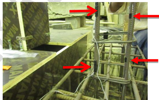
Figure 3: Strain Gauge locations
