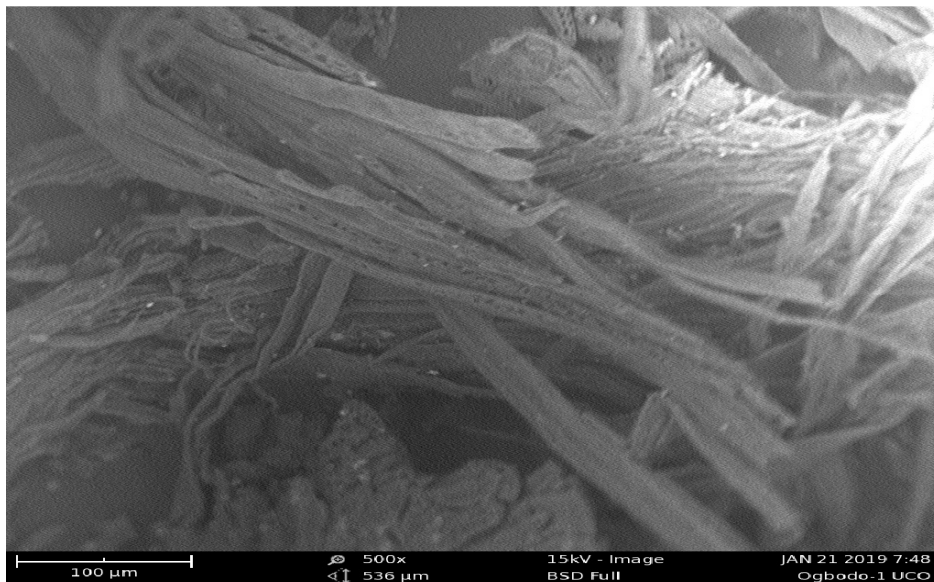
Fig 1: SEM image of un-carbonized ogbono shell @ 100µm
