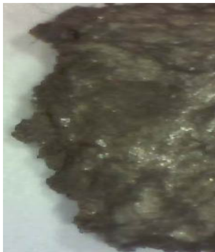
84 85 Figure 1. Pb:Sn:Bi alloy with carbon particles
