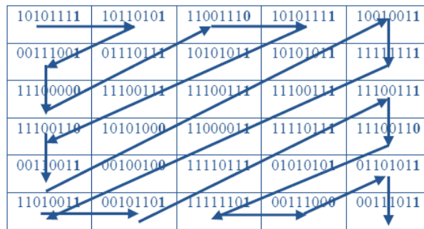
Fig 2: Basic Zigzagging Scanning process
