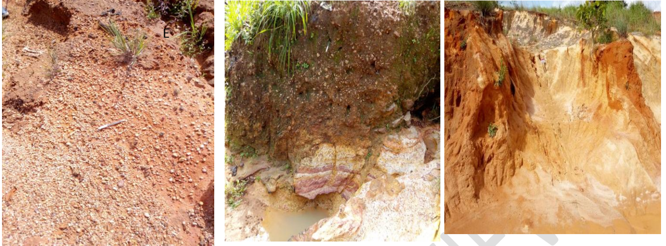
Plate E= Pebbles, F = Sandstone with a sharp contact of kaoline and G= Sand
