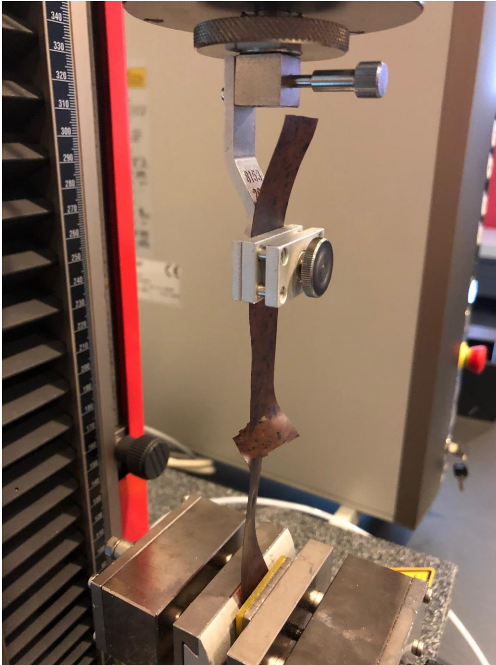
FIG. 2 Image of the set-up for tensile testing (one of the “glass samples”)
